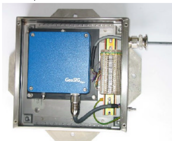
Figure 2. A view from an ISPE sensor with stainless steel housing.
