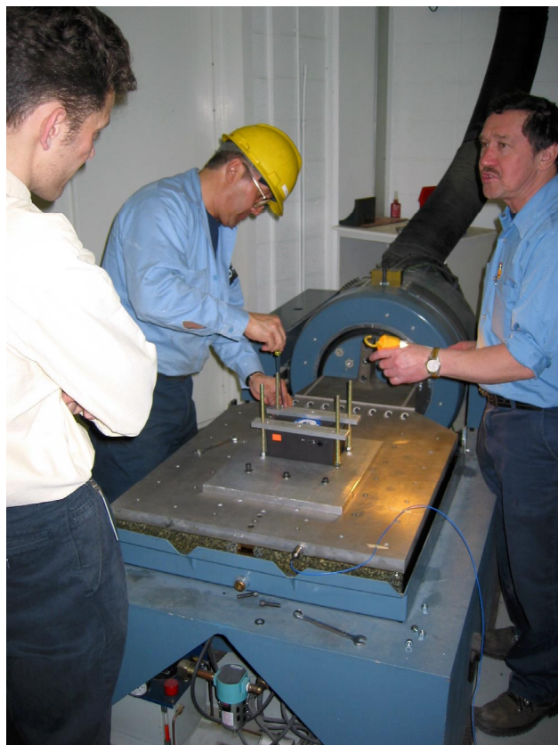
Figure 3. IREQ Shake Table testing of the IA-1 prototype
