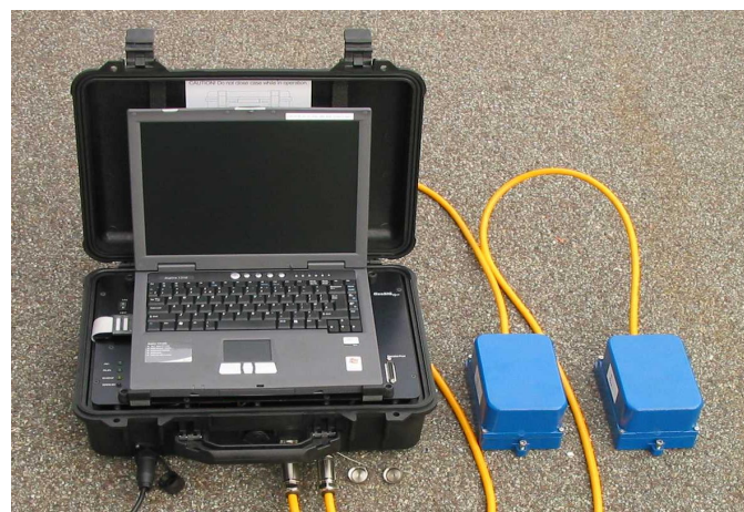
Figure 1. The new GSR-12/16PC Recorder with two sensors attached
