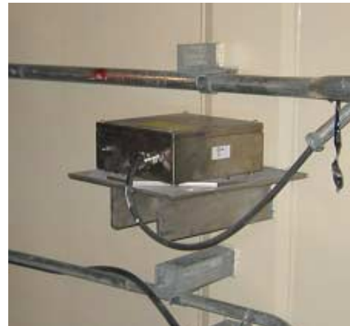
Figure 18. Field accelerometer, customer installation.
