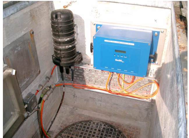
Figure 7. Recorder at freefield station on bedrock (F2).
