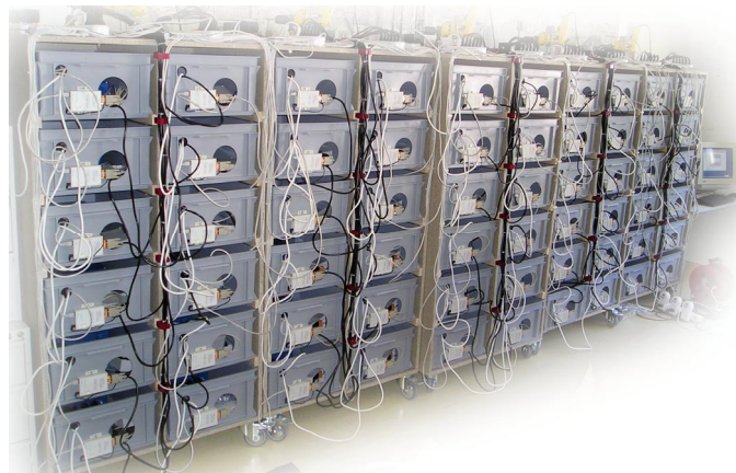
Figure 5. Burn In Cabinets
