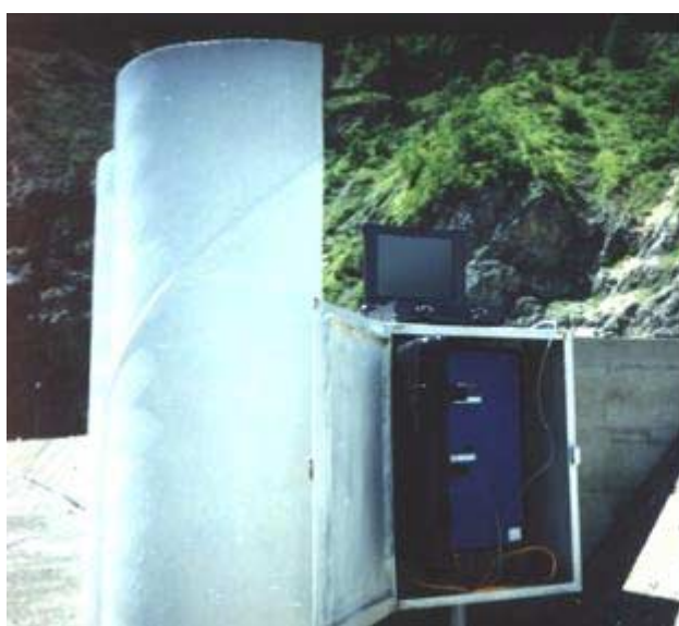
Figure 5. One of the Strong Motion Instruments.
