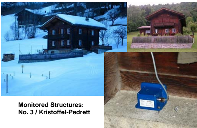
Figure 11. VE-33 installation horizontal on a foundation wall.
