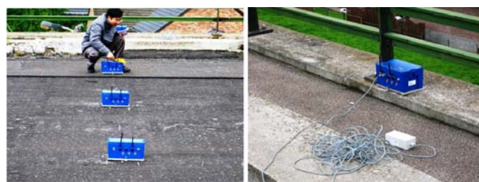
Figure 4. GMS-18 in operation (left) and the master unit with the GPS time synchronization module attached (right) .
