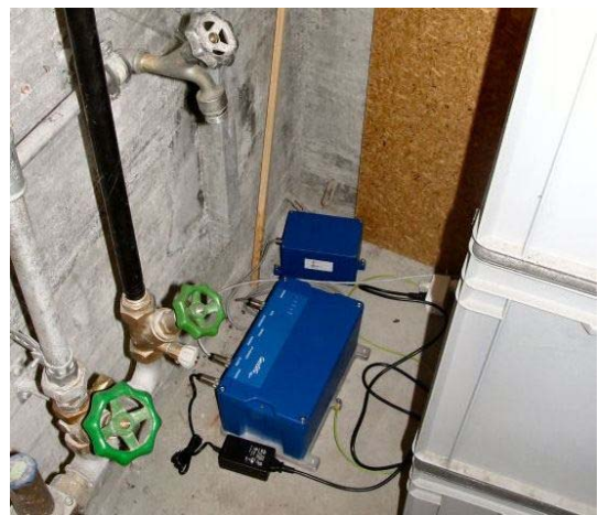
Figure 4. GeoSIG GMS and sensor installed in a basement
