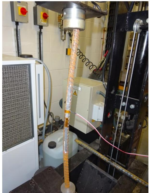
Figure 4. Rebar at a Strain of 2040 $\mu$  $\epsilon$
