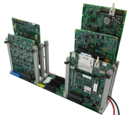
User-replaceable modular plug-in electronic boards make nair extremely maintainable and future-proof
