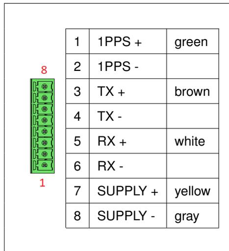
Table 11: fora-OVP-IN PWR GPS pinout
