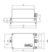
Cast aluminium, sealed access cover 195 x 112 x 95 mm IP65 optional IP68 - 30 °C to + 85 °C - 30 °C to + 85 °C 0 % to 100 % (non-condensing) Floor mounted Single bolt, surface mount, adjustable within ± 3 °
