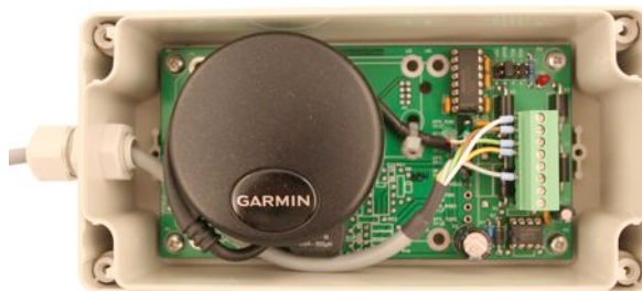
Figure 12. Inside view of the GXR-GPS housing
