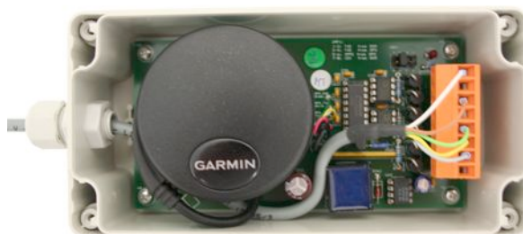
Figure 13. Inside view of the GXR-GPS-485 housing
