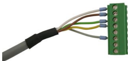
Figure 4. Connector wiring GXR-GPS
