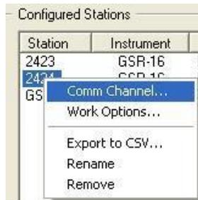
9. Change the connection type to a dial-up connection through a dedicated modem and choose the correct COM port (the one where the GSM modem is connected), also set the connection speed to 19'200 and enter the appropriate phone number for the GSM. The recommended (default) modem init string in GeoDAS is AT&F0E0V1X1S0=0
