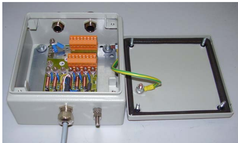
Figure 2. Interconnection Junction Box (150 x 150 x 80 mm)
