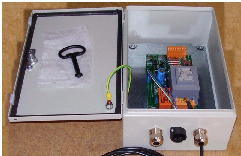
Figure 5. Central Communication Box (300 x 200 x 120/140 mm)
