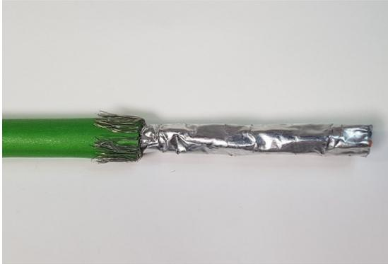
Figure 17. Fold back the cable shield
