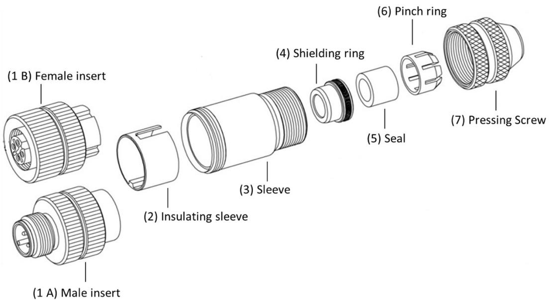
Figure 11. Internal view of Binder Connector
