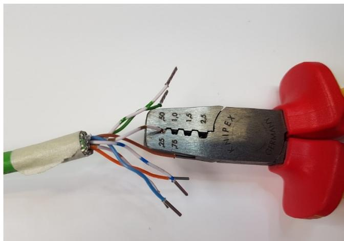
Figure 24. Crimping end sleeves
