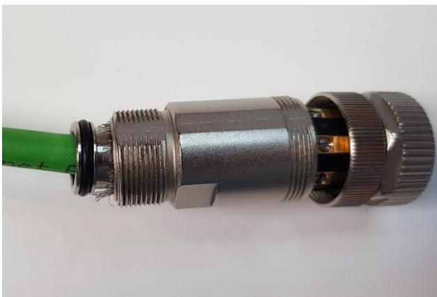
Figure 31. Pushing the shielding ring into the sleeve
