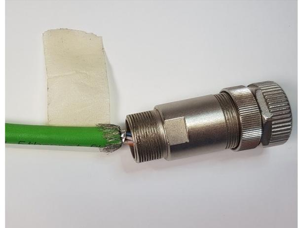
Figure 28. Removing the tape
