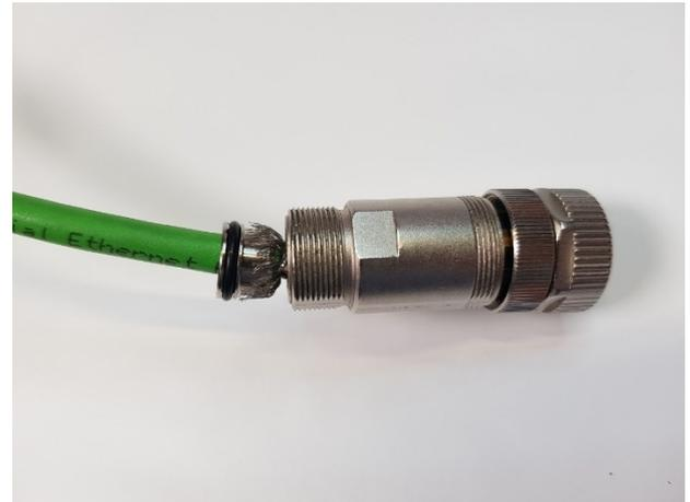
Figure 30. Bending the shield onto the ring
