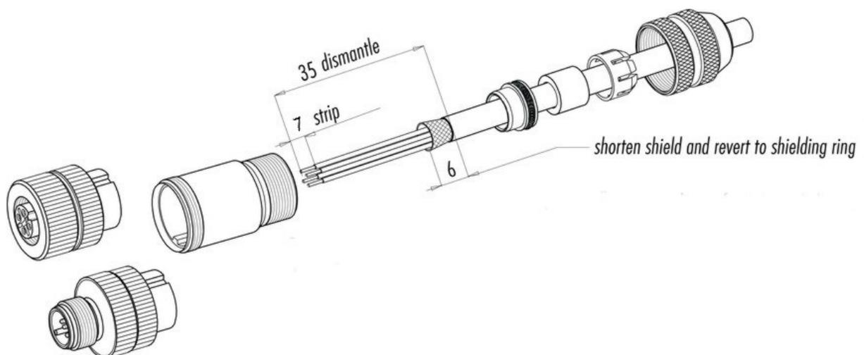
Figure 12. Preparation of the connector, insert cable
