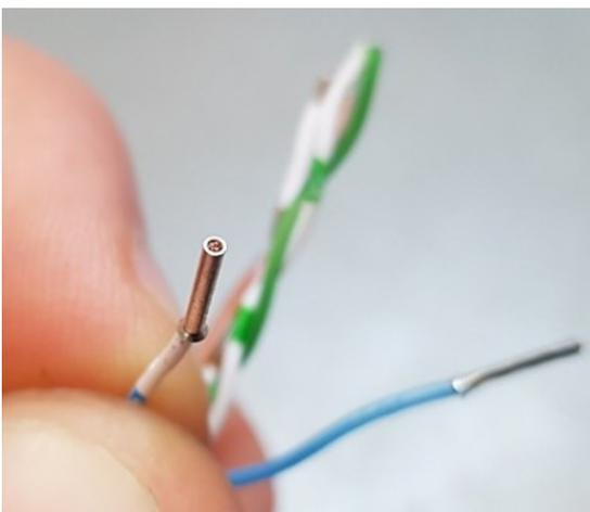
Figure 23. End sleeve with copper visible
