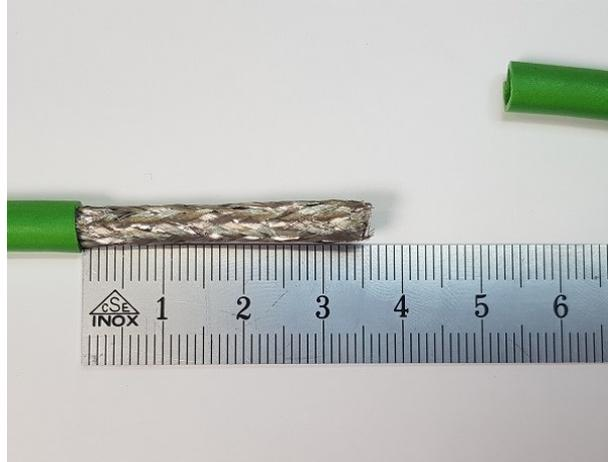
Figure 14. Remove 35mm of the cable jacket
