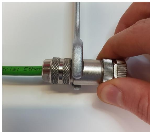
Figure 35. Tightening with wrench
