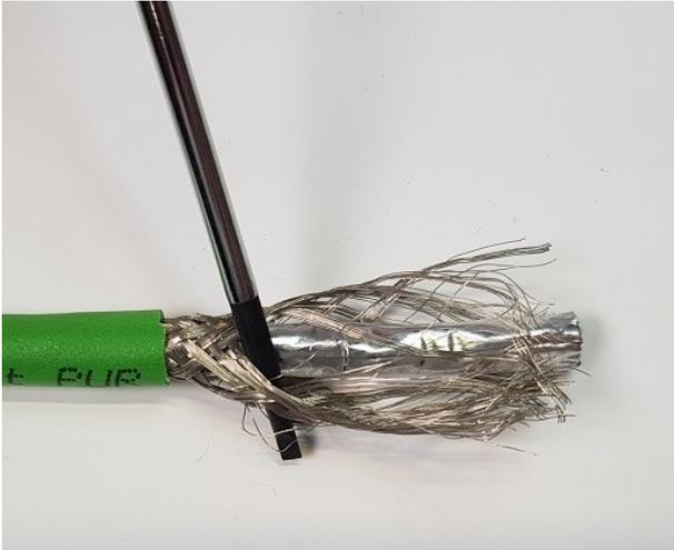
Figure 15. Unravel the cable shield
