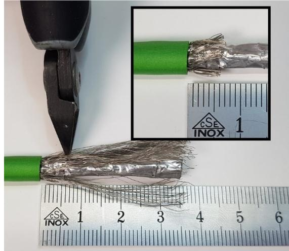
Figure 16. Shortening the shield to 6mm
