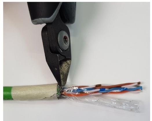
Figure 20. Cut off plastic foil
