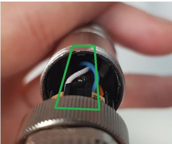
Figure 34. Alignment of guiding groove
