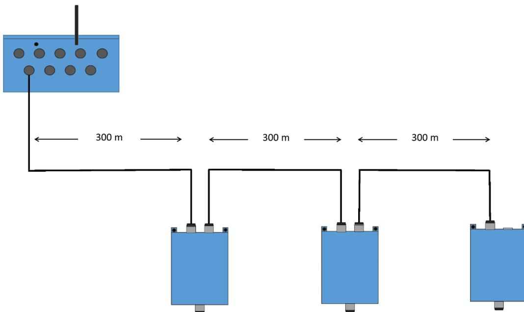
Figure 3. 3 sensors cable configuration
