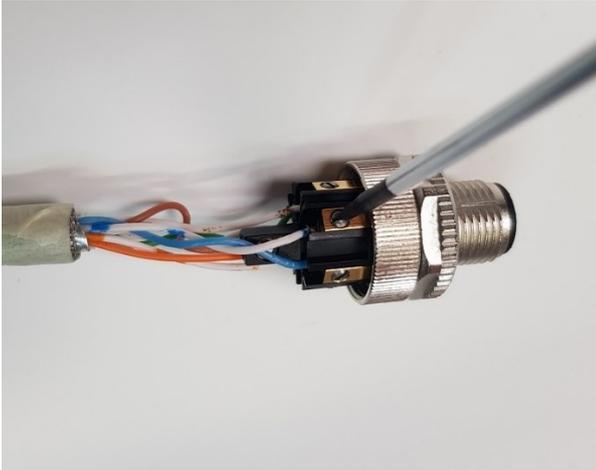
Figure 25. Screwdriver applied on pin1 of the male connector
