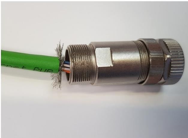
Figure 29. Pushing out the wire strands
