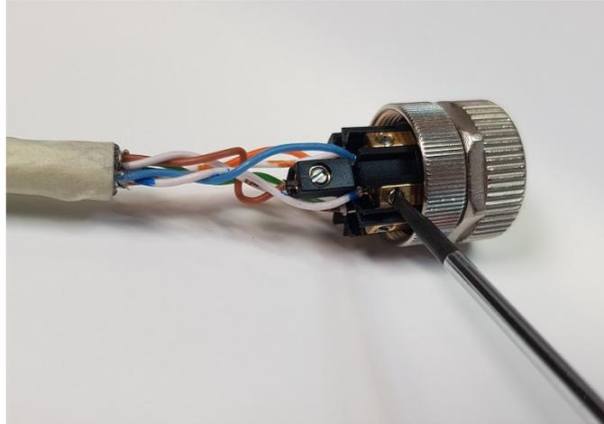
Figure 26. Screwdriver applied on pin1 of the female connector
