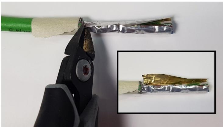
Figure 19. Cut off aluminium foil
