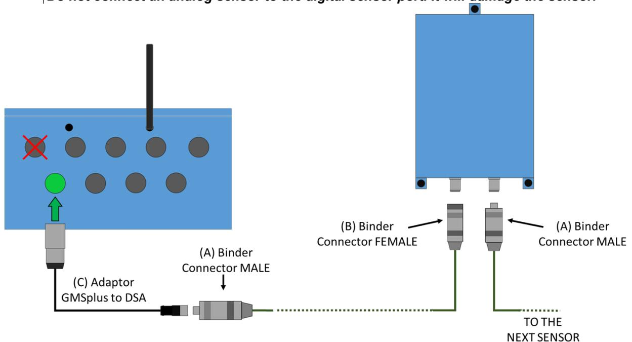
Figure 9. Sensor cable wiring diagram, general overview
