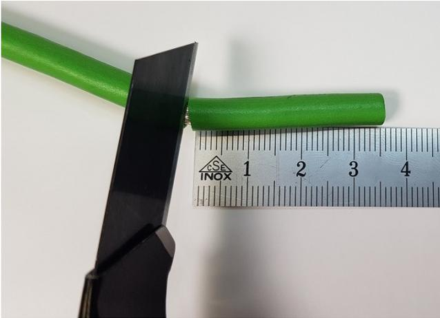
Figure 13. Cut 35mm of the cable jacket
