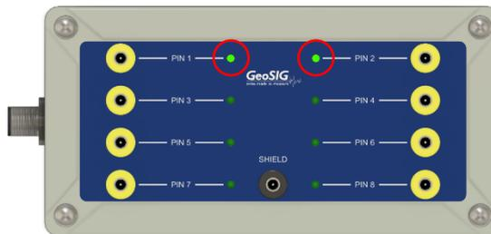
Figure 44. Shortcut between PIN 1 and PIN 2.
