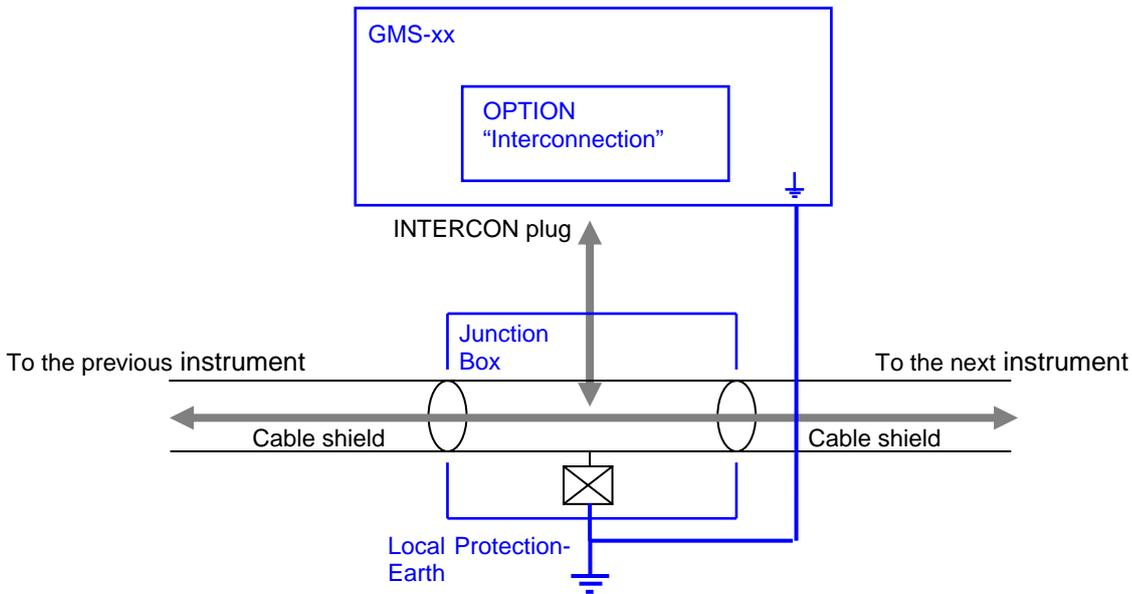
Figure 2. Wiring, including *Interconnection Junction Box*
