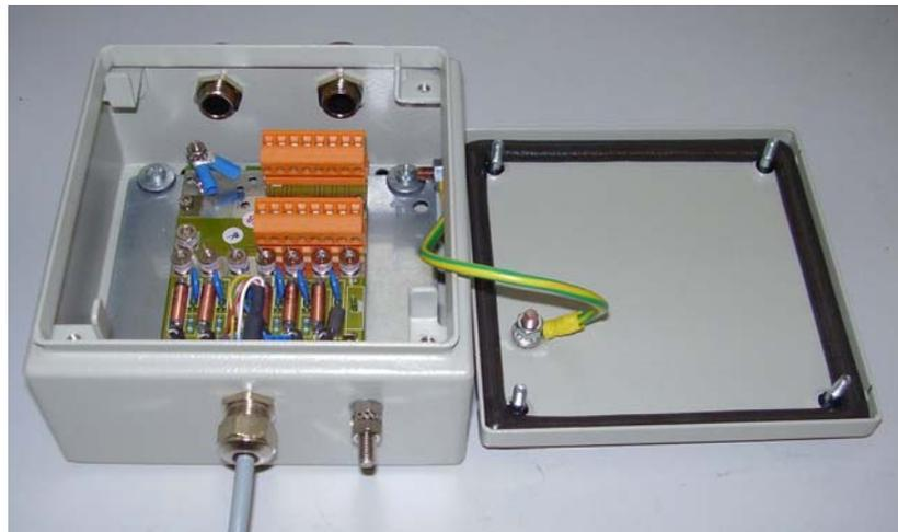
Figure 1. *Interconnection Junction Box* (150 x 150 x 80 mm)
