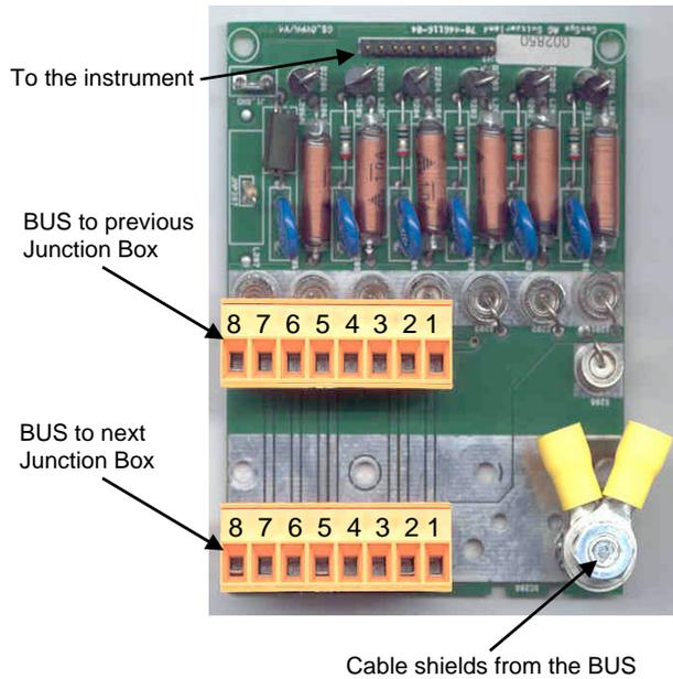
Figure 4. Connectors inside Junction Box
