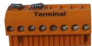
Figure 6. Termination Connector
