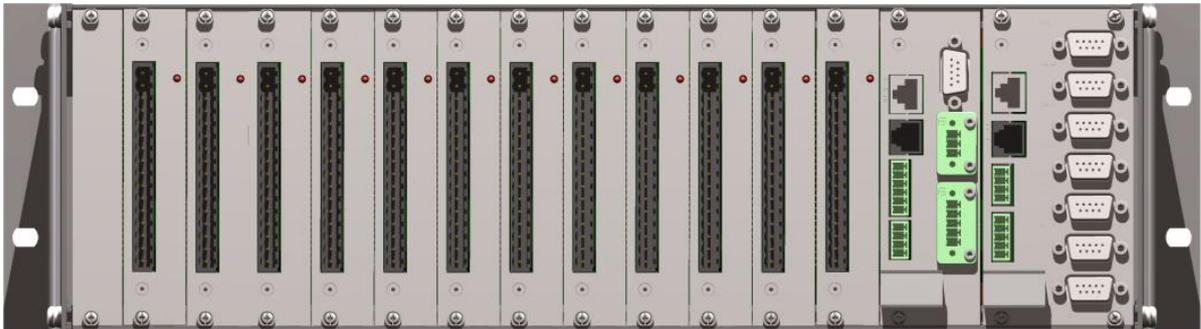
Figure 5. Back view of the CR-6-BASE Base Rack
