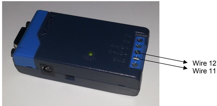
Figure 2, MOXA TCC-80I interface for RS-485
