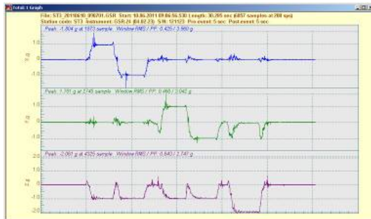
Fig 6. AC-63 2 g tilt-test
