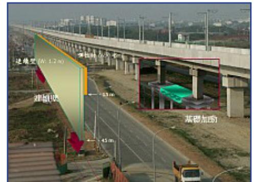
Planning the foundation-stiffening blocks and the underground wave-barrier-wall.
