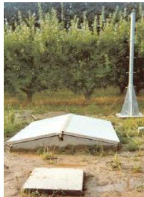
The earthquake early warning system includes 24 stations housing AC-23 accelerometers, set every 10 km apart, which transmit data and alarms to a central sign posting unit in Marseille.
