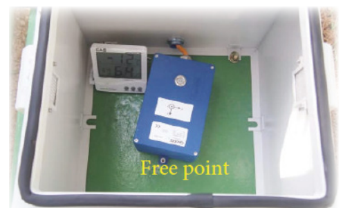
Accelerometers installed at roof point (above) and free point (below).
