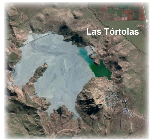
Las Tórtolas is a flotation plant located 45km from Santiago at about 750m above sea level. This complex also includes a tailings dam, which is used to store byproducts of mining operations. Satellite image (above) and map (below) by Google maps.
