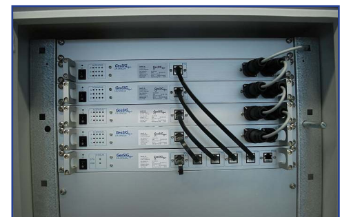
The CR-5P central recording unit integrates the digitiser board and an industrial PC in one platform.
