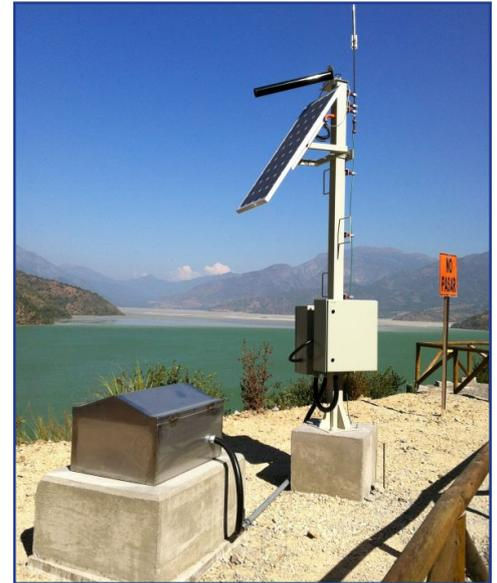
Solar panels were also set up with large-capacity batteries to power the GSR-18 units with AC-63 accelerometers synchronised with GPS timing.
