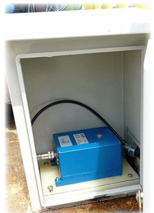
AC-73 accelerometers sense vibration, and the data is sent to GMSplusD and GeoDAS to determine exceedances.
