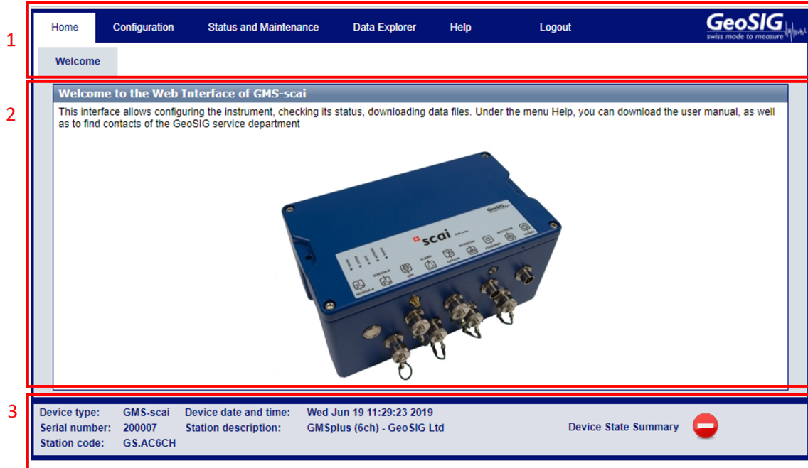
Figure 32: The home panel of the web interface
