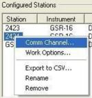
9. Change the connection type to a dial-up connection through a dedicated modem and choose the correct COM port (the one where the GSM modem is connected), also set the connection speed to 19'200 and enter the appropriate phone number for the GSM. The recommended (default) modem init string in GeoDAS is AT&FEOVIX1S0=0
