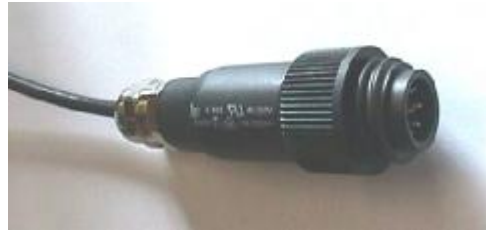
Binder 7p male connected to GPS
