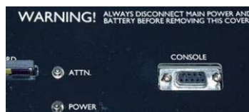
Figure 6: Internal RS-232 connector for the console
