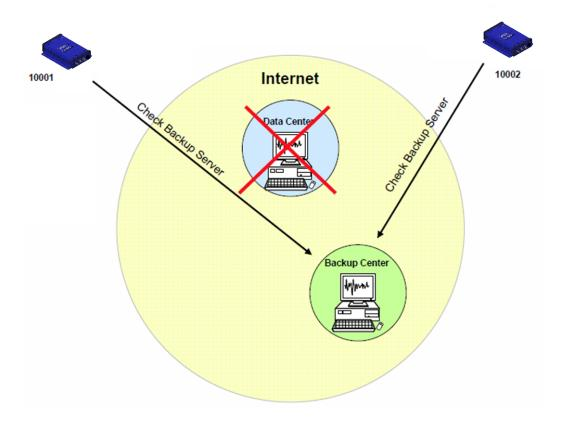
Figure 23: Connection to backup server in case connection to main server fails
