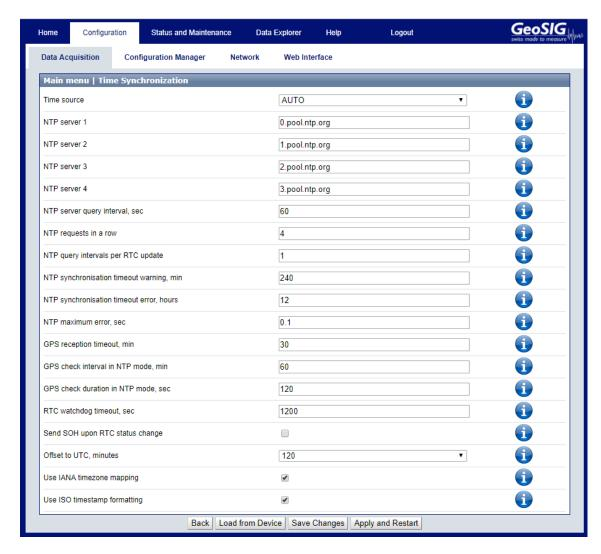
Figure 67: Edit Time synchromization Parameters
