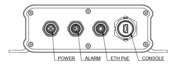
Figure 2: Instrument with all connectors. Antennas are not mounted
