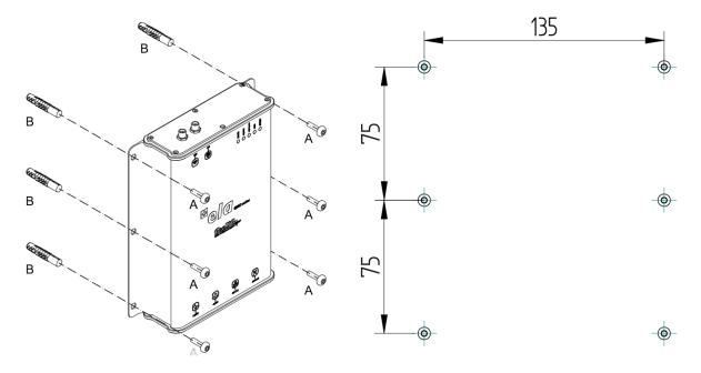
Figure 4: Direct installation on wall or floor
