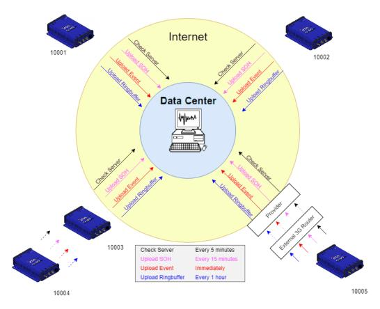
Figure 19: Normal operation in a network
