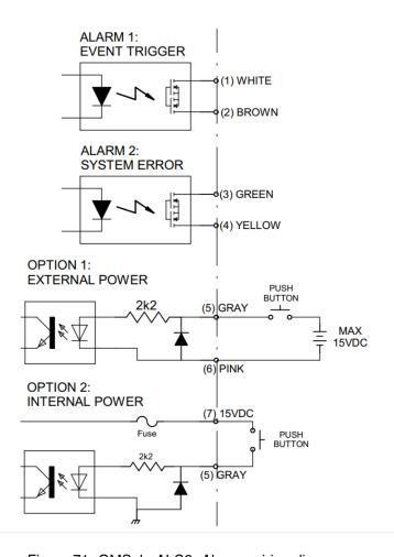
Figure 71: GMSela-ALC2: Alarms wiring diagram
