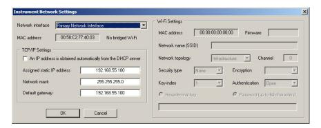
Figure 27: Configuration of wired Ethernet
