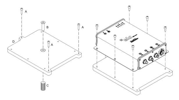
Figure 5: Installation with the base plate
