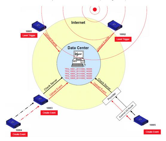
Figure 21: Behaviour on Events: Upload of extracted events
