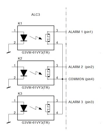
Figure 72: GMSela-ALC3: Alarms wiring diagram
