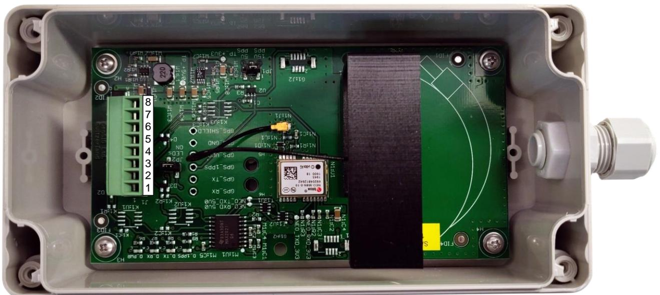
Figure 4. Inside view of the GXX-GPS housing
