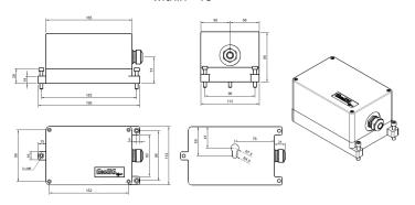
Standard AC-23 floor mounted, full scale  $\pm$  2 g, 2 m cable with cable inlet and recorder mating connector, concrete anchor bolt and user manual on CD
