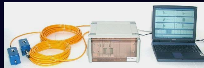
Portable CR-4, complete with sensors
