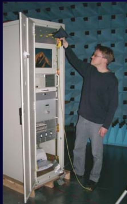
Full size CR-4, under EMI testing
