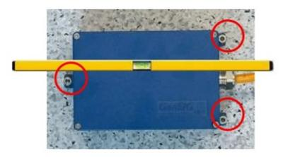
• Adjust the levelling with the spirit level in y-direction
