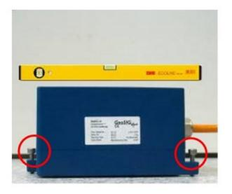
• Adjust the levelling with the spirit level in x-direction
