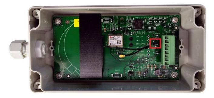
• The PCB is equipped with 4 LED's to indicate the GMS-TIM signal status
